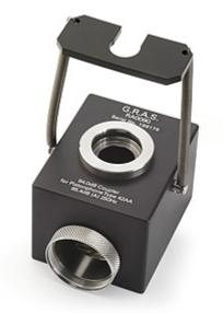
A larger-volume coupler for enabling GRAS 42AA/AP Pistonphone to produce a sound pressure level of 94 dB instead of 114 dB re. 20 Pa. Essential when calibrating highly sensitive, GRAS low noise measuring systems.
