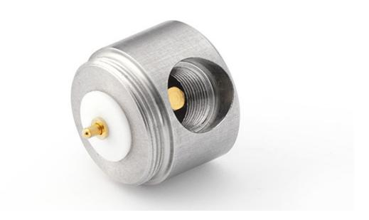
Length: 10 mm Inner threading for preamp.: 5.70-60 UNS-2 Outer threading for mic.: 11.70-60 UNS-2 Material: stainless steel The RA0001 is a right-angled adapter for using a 1/2" microphone with a 1/4" preamplifier. It can be used with any standard 1/2" microphone and 1/4" preamplifier such as the GRAS 26AC. The RA0001 could be useful in situations where the microphone has to be flush mounted on a wall.
