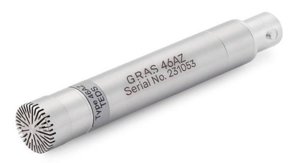
Freq range (±3 dB): 0.5 Hz to 20 kHz Dyn range: 17 dB(A) to 138 dB Sensitivity: 50 mV/Pa Use: For low frequency acoustic diagnostics The GRAS 46AZ is a 1/2" Constant Current Power (CCP) free-field microphone set for measuring medium sound pressure levels at low frequencies. It is terminated with a BNC connector and is TEDS compatible. The equivalent traditional 200 V (LEMO) type is <u>GRAS 46AN</u>.
