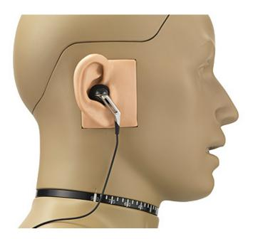
Connection: Traditional Power Supply (200 V/LEMO) Channel(s): 2 ANSI: S3.36, S3.25 IEC: 60318-4 ITU-T Rec. P.57 Type 3.3, based on ITU-T Rec. P.58 The 45BB-9 KEMAR is a manikin configured with externally polarized ear simulators and anthropometric pinnae for dual-channel ear- and headphone test. Its corresponding CCP equivalent is the <u>GRAS 45BB-10</u> <u>KEMAR with Anthropometric Pinnae for Ear- and</u> <u>Headphone Test, 2-Ch CCP.</u>
