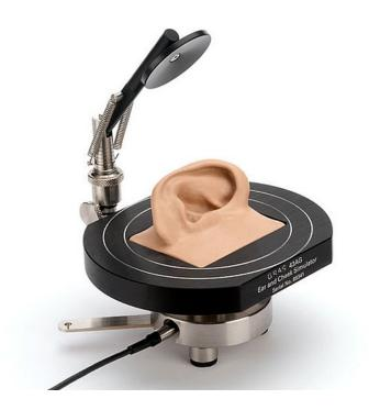
ANSI: S3.7 IEC: 60318-4 Other specs: Refer to the ear simulator included in the specific configuration The GRAS 43AG Ear and Cheek Simulator represents the section of a head most important for realistic reproduction of the acoustic properties of the ear of an average human head. It allows the use of an ITU-T type 3.3 pinna or an Anthropometric Pinna, either with an IEC 60318-4 Ear Simulator, a Low-Noise Ear Simulator system, a High-Frequency Ear Simulator or a Hi-Res Ear Simulator.
