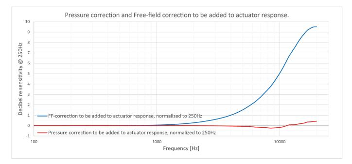
The corrections from actuator to the real pressure and free-field responses
