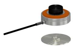
When the microphone is placed over the mounting disc, a center guide ensures that the microphone will be attached and centered to the disc correctly once the magnetic force kicks in. In this way, it is easy to mount in difficult-to-access locations with no loss of placement accuracy.
