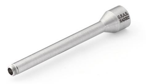
Length: 39 mm Inner threading for preamp.: 5.70-60 UNS-2 Outer threading for mic.: M3 Material: stainless steel The GRAS RA0082 is an adapter for using a 1/8" microphone with a 1/4" preamplifier.
