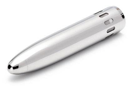
Length: 17.4 mm Outer diameter: 3.5mm Threading (mic. protection grid threading): M3.175x0.2 Material: Stainless steel Weight: tbd The RA0173 is specially designed and optimized for use with 1/8" microphones for sound pressure measurements, when high speed wind comes from one known direction e.g. in a wind tunnel.
