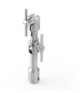
Material: Stainless steel Dimension: For 7 mm Special feature: Adjustable in 45 degree steps The GRAS RA0096-S1 is an adapter for mounting a microphone set (microphone/preamplifier) on tripods having a standard 1/4" UNC-20 male thread. The adapter is provided with a clamp for attaching a 7mm diameter preamplifier. The microphone can be set in angles between 0 and 180 degrees in 45 degree steps.
