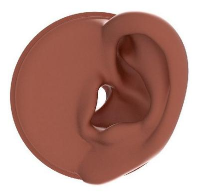
Anatomically shaped concha and ear canal Improved fit and repeatability Outer pinna with improved collapsability Resilient mounting KB5011 is a left anthropometric pinna for 45CA for accurate and repeatable testing of headphones and earphones. It has anatomically correct ear-entrance and ear-canal with correct soft ear helix and provides perfect sealing and insertion accuracy for headphones and earphones. The hardness is 35 Shore 00
