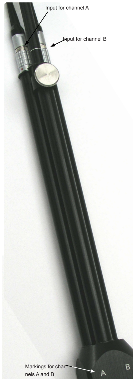
Fig. 2.1 Showing the inputs and markings for the two preamplifier inputs
