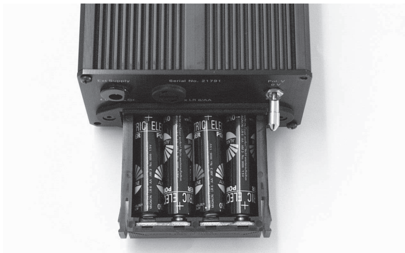
Fig. 3.1 Battery drawer open: note polarity of batteries
