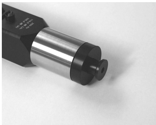
Fig. 3.5 1/8-inch microphone adapter inserted in the coupler
