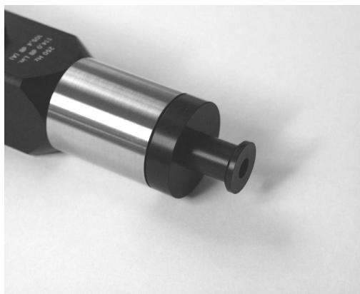
Fig. 3.4 1/4-inch microphone adapter inserted in the coupler
