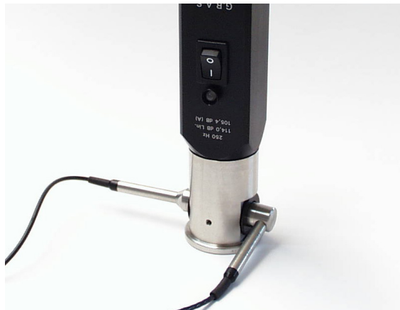
Fig. 4.1 Two-port Coupler RA0024 shown here with the two phase-matched microphones of an intensity probe
