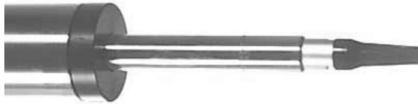
Fig. 3.3 1/2-inch microphone inserted in the coupler
