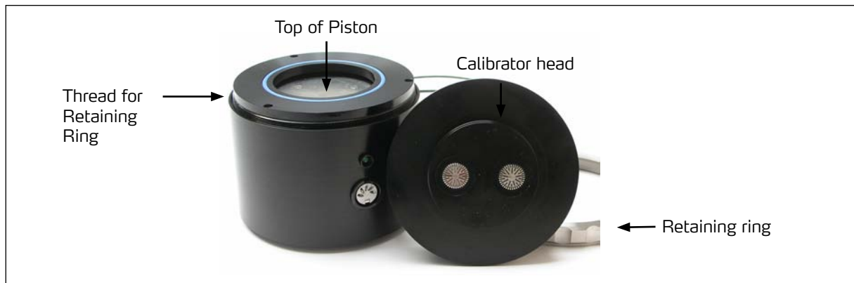
Fig. 4. The Calibrator Head removed to expose top of piston, the Calibrator Head, and flush-mounted microphones.
