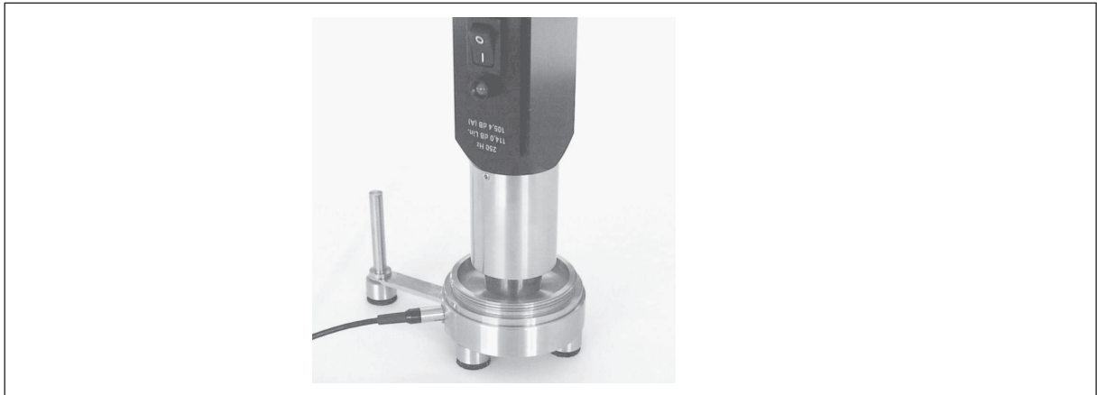
Fig. 4. Calibration using the Pistonphone a) Place coupler over microphone, push gently down to microphone stop b) Switch on
