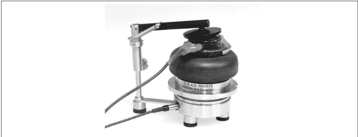
Fig. 2. Example of a supra-aural earphone mounted on the test jig
