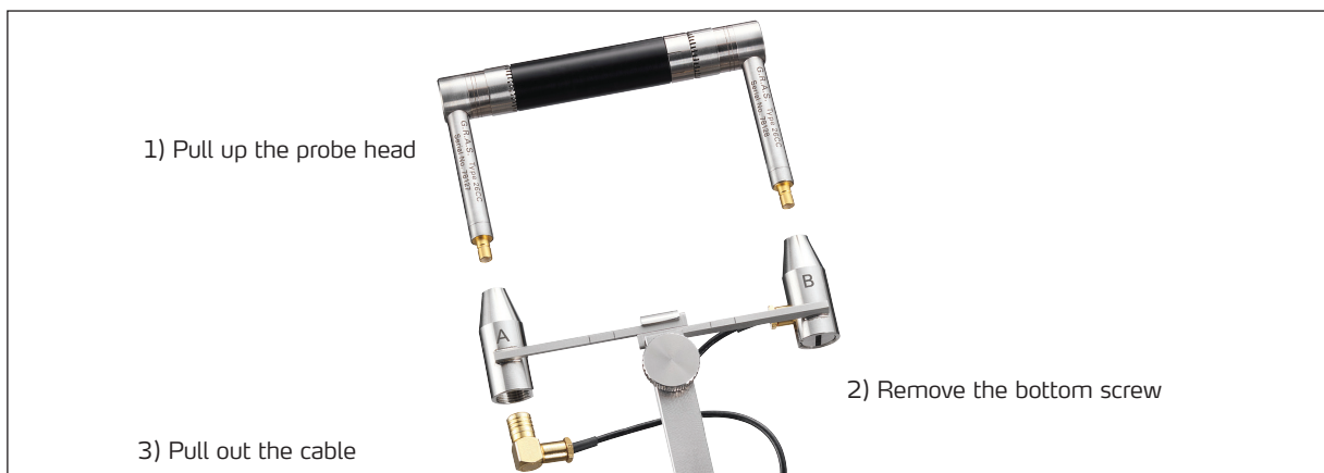
Fig. 8. Releasing the cable connectors from the holder assembly
