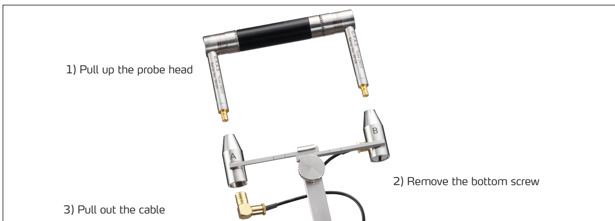
Fig. 7. Releasing the cable connectors from the holder assembly.
