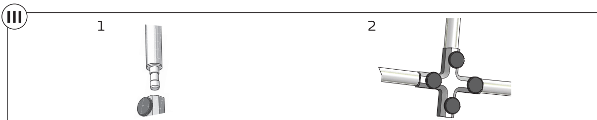
Fig. 24. Attaching vertical poles to the B-layer circle.
