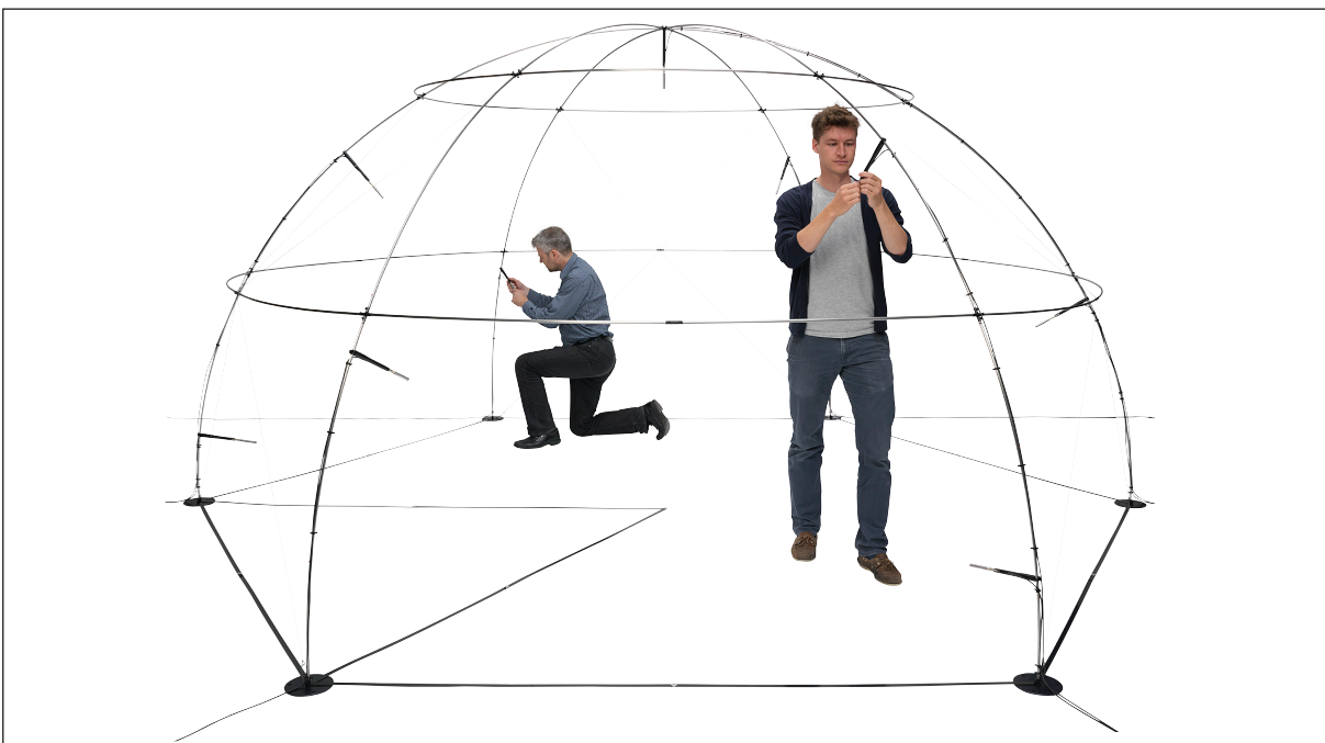
Fig. 10. The structure being mounted with microphones and cables for a 10-channel setup.
