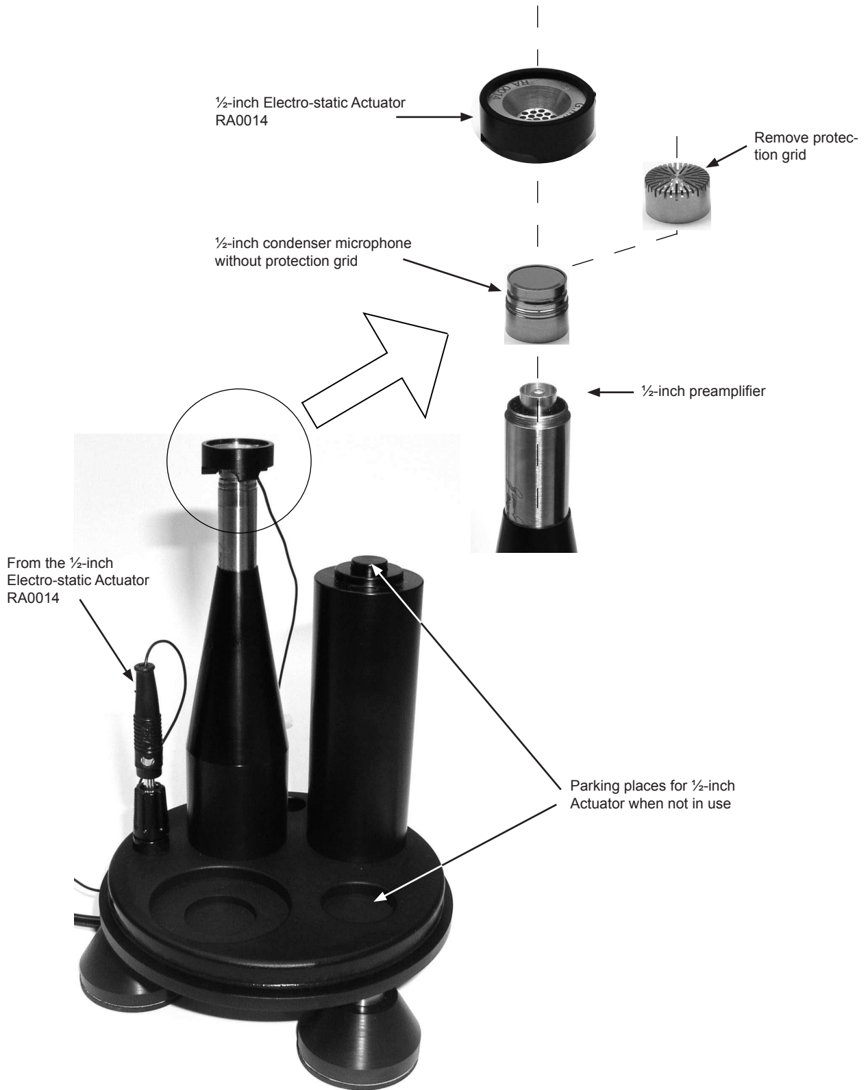
Fig. 3 Set-up for calibrating the frequency response of a 1/2-inch condenser microphone
