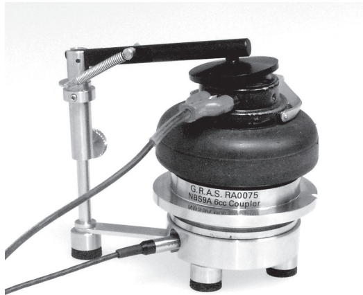
Fig. 6.2 Example of a supra-aural earphone mounted on the test jig
