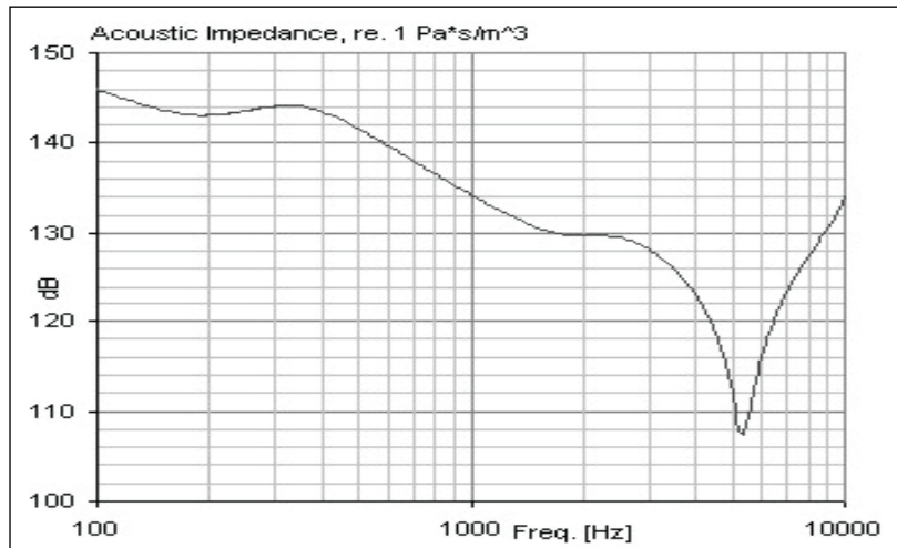
Fig. 9.2 Type RA0039 acoustic input impedance
