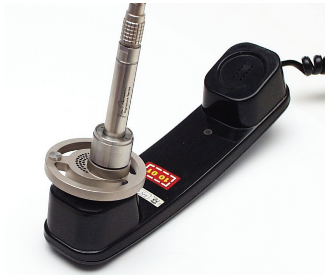
Fig. 11.3 Place the Pinna Simulator centrally over the earpiece of the telephone handset
