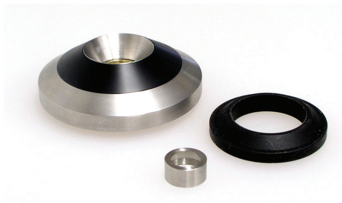
Fig. 9.1 IEC 318 Ear Simulator Type RA0039 as delivered
