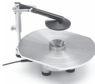
Fig. 1.2 Type 43AA shown with mounting plate GR0339 for testing ear-phones fitted with fluid cushions
