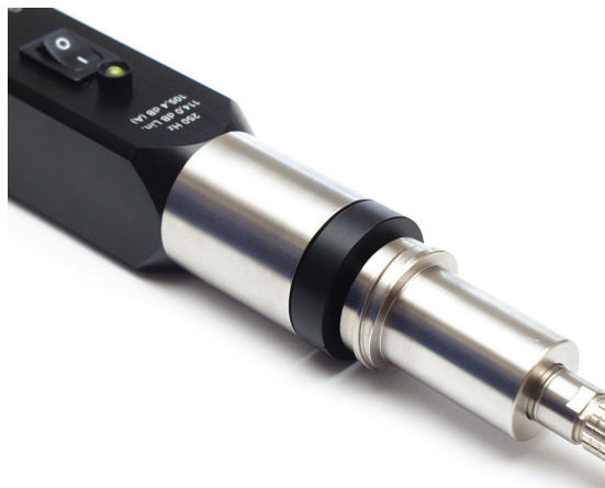
Fig. 4.6 Gently push the microphone into the Pistonphone's coupler until it reaches the stop
