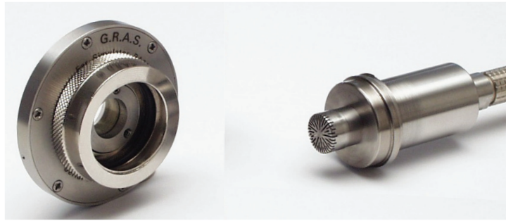
Fig. 4.5 Showing the two halves of the snap coupling to give quick access to the microphone
