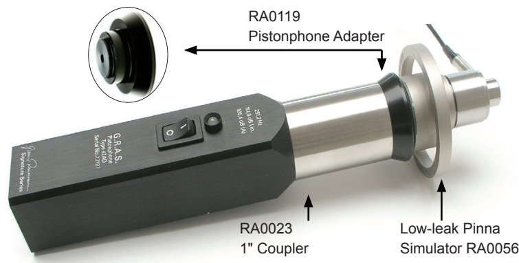
Fig. 5.4 Calibration-check set-up. Make sure that the rubber seal of the Pinna Simulator seats firmly inside the Pistonphone Adapter
