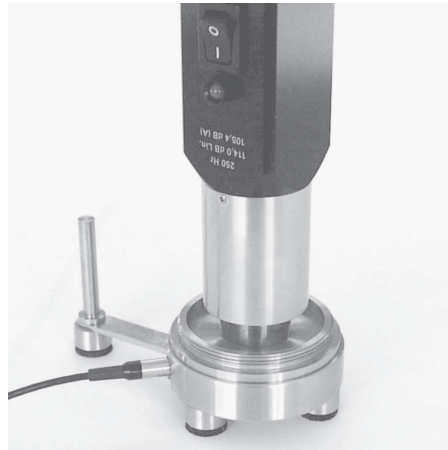
Fig. 6.4 Calibration using the Pistonphone
