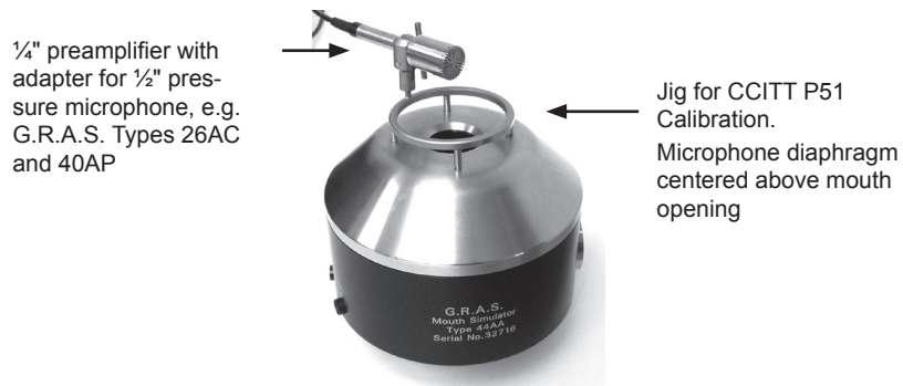
Fig. 13.8 Set up for calibrating the Mouth Simulator according to CCITT P51
