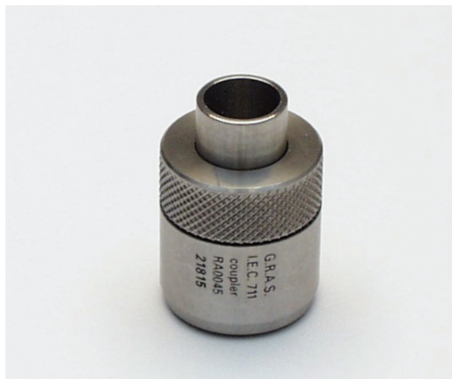
IEC 60711 Ear Simulator Type RA0045
