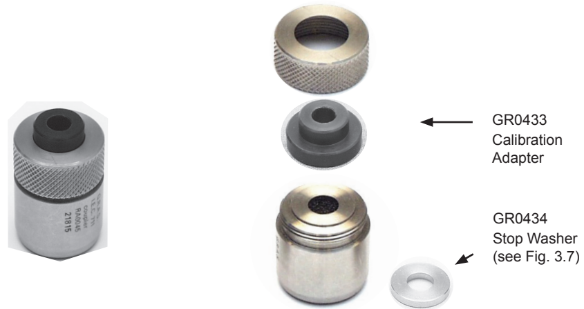
Fig. 3.6 Assembled and exploded views of the coupler itemising user-serviceable accessories for individual calibration
