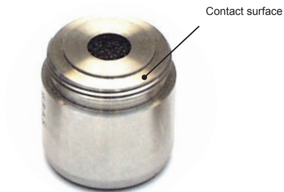
Fig. 10.4 Showing where to apply a thin film of petroleum jelly to improve sealing within a 1" Pistonphone coupler
