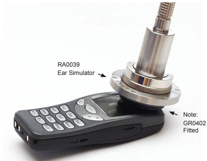
Fig. 4.4 Place the Artificial Ear centrally over the earpiece of the mobile 'phone
