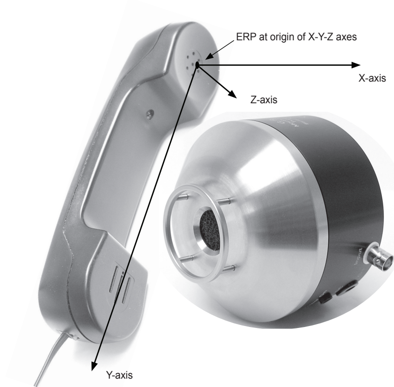
Fig. 13.4 Showing the basic configuration for testing the microphone of a telephone handset. The ear piece lies in the plane of the Y-Z axes. See Fig. 13.5 for geometrical details
