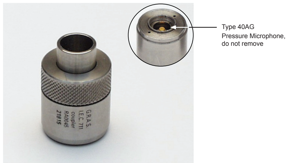
Fig. 10.1 IEC 60711 Ear Simulator Type RA0045 as delivered
