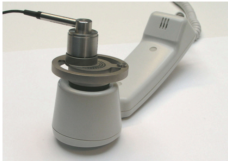
Fig. 5.3 Place the Ear Simulator centrally over the earpiece of the telephone
