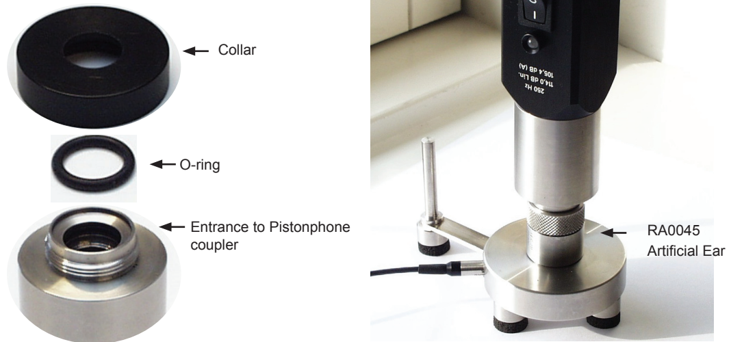
Fig. 3.3 Calibration using the Pistonphone
