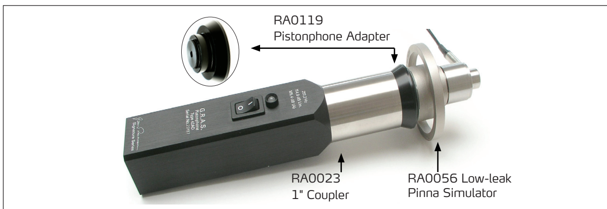
Fig. 5. Calibration-check set-up. Make sure that the rubber seal of the Pinna Simulator seats firmly inside the Pistonphone Adapter
