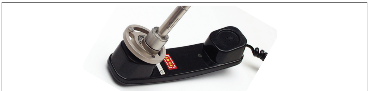
Fig. 4. Place the Pinna Simulator centrally over the earpiece of the telephone handset
